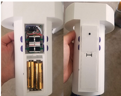
All of the electronics are securely hidden in a separate compartment with a lid held by a screw to make it more difficult to access by typical users.
