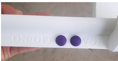
There are two buttons on this side; one to turn the model on and off and the other button to choose between three volume settings.
