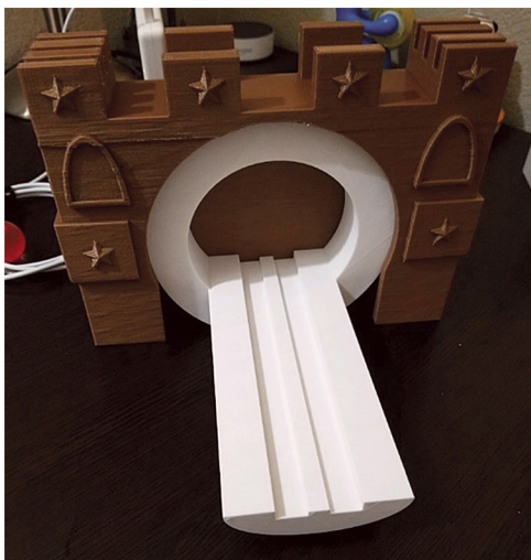
3D-printed shell which looks like the castle cover. This shell can be easily placed over the machine for patients who will be scanned by the pediatric MRI machine.
