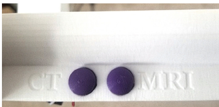
These two buttons function to play sounds to replicate a CT machine, and the other plays sounds to replicate an MRI machine.
